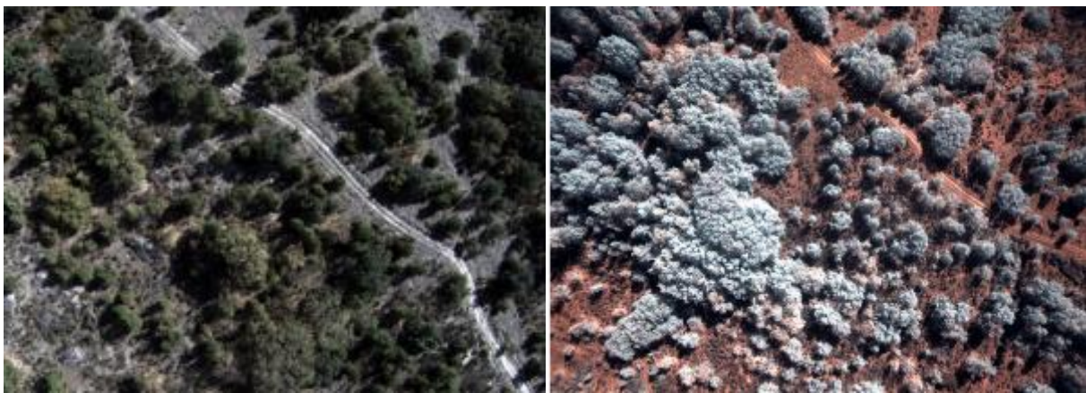
Figure 5 Sample RGB image taken with VIS camera (left) and NIR image taken with NDVI camera (right)
